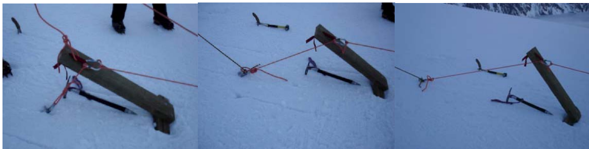
Simulated belayer in the system. From left to right. 0.0 m, 0.5 m, 1.0m back from belay point. All photos were taken at point of failure
